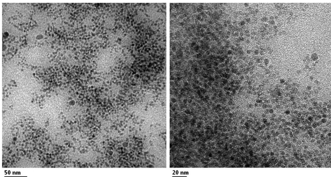
FIG. 1. Transmission electron microscopy images show iron oxide cores of 4–5 nm. The coating material separates the particles but is not visualized because of the lack of electron density of *meso*-2,3-dimercaptosuccinic acid for detection with TEM. The particles are well separated and do not aggregate.
