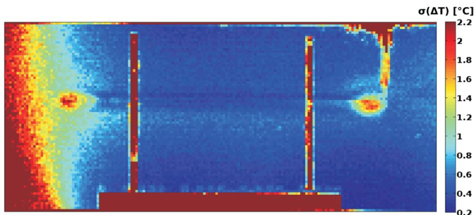
FIG. 5. Map of mean SD, calculated from the set of phase-contrast images for every pixel separately, and translated into temperature values.
