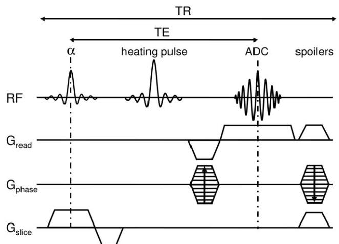
FIG. 2. GRE sequence including an off-resonant heating pulse as used in the thermometry experiments.
