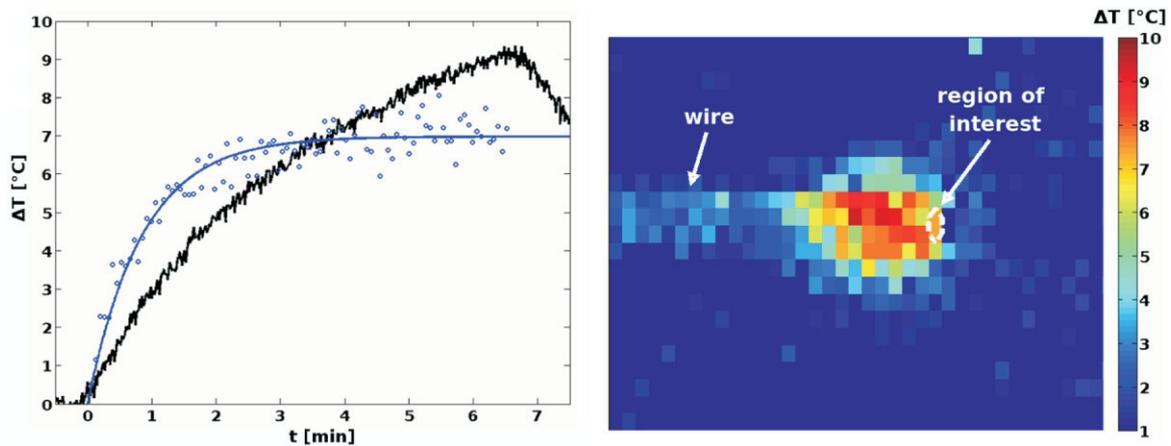
FIG. 4. Left: Temperature from the MRI temperature maps averaged over a two-pixel region of interest (blue line) in comparison to the readings from the fluoroptic probe (black line). The MRI measured temperature distribution near the wire tip is depicted on the right. The temperature was averaged over the two pixels in the region indicated by the white dotted line (approximately 4 mm beyond the tip of the wire).
