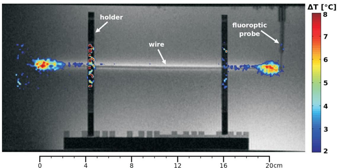
FIG. 3. Overlay of a scout image and the PRF shift temperature map after the 7-min heating period. Both images were interpolated to a matrix size of  $384 \times 1024$  (two-fold interpolation of the scout and four-fold interpolation of the temperature map). Only temperature differences larger than  $2^{\circ}\text{C}$  and in an area 20 mm adjacent to the wire are shown. Pronounced hot spots are visible at both tips of the wire.
