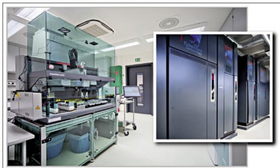
Fig. 2: Pipet-roboter to generate small cryo-tubes from routine blood vials and fully automated -80^{\circ}\text{C} cryo-repositories for the long-term storage of about 1.1 Mio cryo-tubes hosted by the ibdw.
