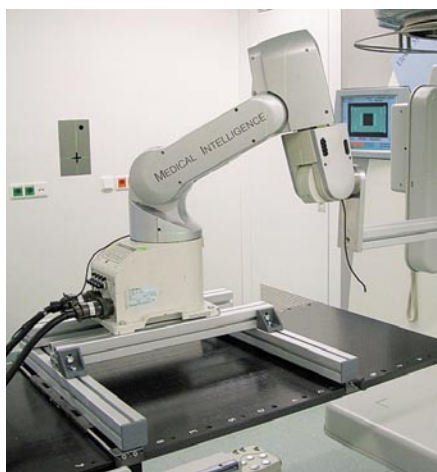
Fig. 2: Test set-up for tracking a moving object in order to keep it within the therapy beam.
