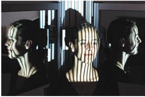
Fig. 2: Stereophotogrammetry with the optical sensor FaceScan3D (3DShape, Erlangen) to generate three-dimensional data of the facial soft parts.
