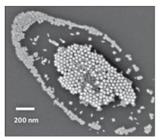
Fig. 2: Scanning electron micrograph of spherical and rod-shaped gold nanoparticles
