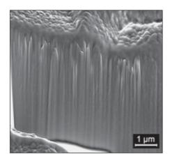
Fig. 1: FIB cut across a silver-doped titanium coating.
