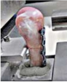
Fig. 2: Experimental fracture model to test angle-stable mini implants at the metacarpals.
