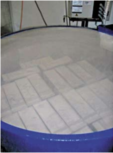
Fig. 2: The stem cells are stored in liquid nitrogen at minus 196 °C.
