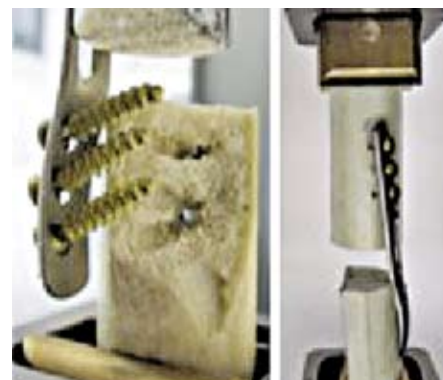
Fig. 1: Biomechanical testing of a newly developed angle-stable external ankle plate.
